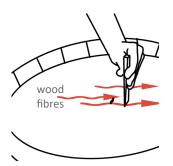
If there is a leak on the drum lid, mark the spot and place a chisel ca. 1 cm behind or in front of the leak at cross-angles to the fibre direction and make a hole using a hammer.
