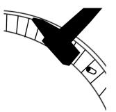
Tap the wooden cone carefully into the hole until it can no longer be driven in any further.
