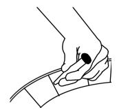
Place the puncture tool to the leaking area.
