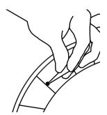
Place the wooden cone in the enlarged hole.
